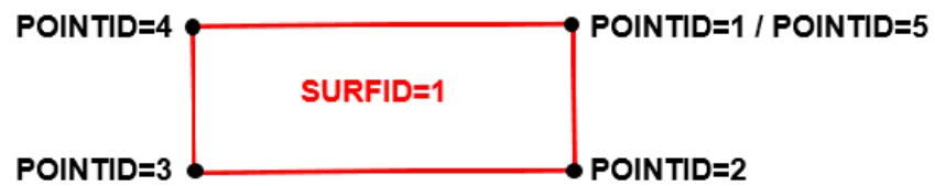
Figure 7: Example for 2D pedestrian shape definition
